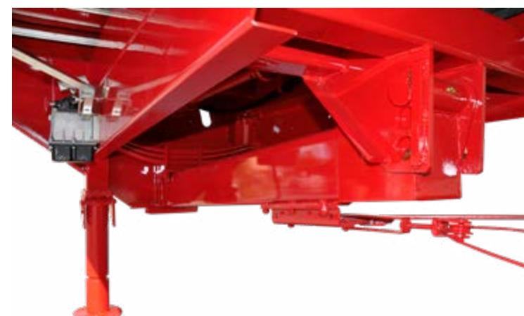
Drawbar with springs of parabolic 2 leaves for the model E87LMP2 and drawbar with springs of parabolic 3 leaves for the models E88LMP2 and E92LMP2 with hydraulic jack-stand with manual pump.
